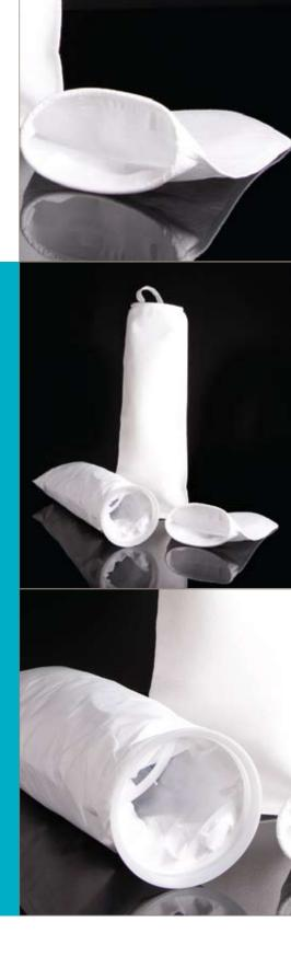
Parker domnick hunter's range of bag filters are manufactured from a variety of filter media each specifically chosen for its compatibility with a wide range of process liquids. Parker bag filters are of a fully welded design rather than sewn. No process liquid can bypass through needle holes caused by the sewing process or around a sewn ring. Parker domnick hunter's range of filter bags include:
